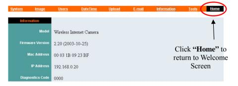
The Information table provides detailed information of the Internet Camera, such as the Model Name, Firmware Version, Mac Address, and IP Address.
